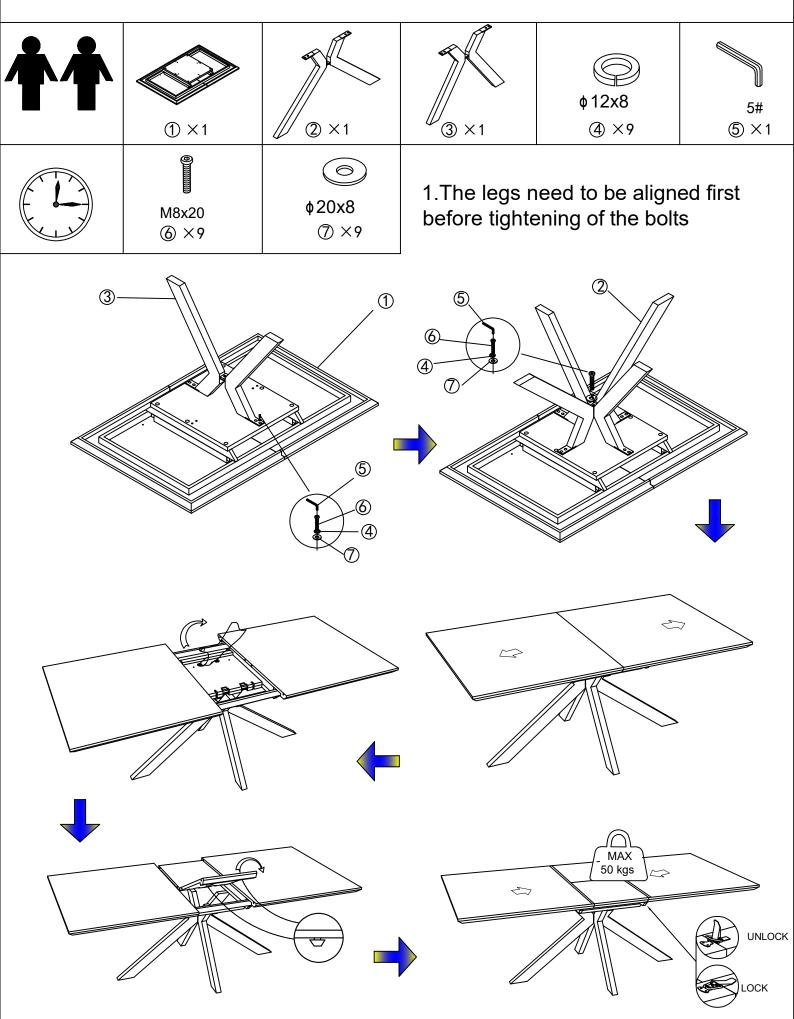
2. Adjuster bolt is (under table frame extension) to line up/level off the table top, if required
