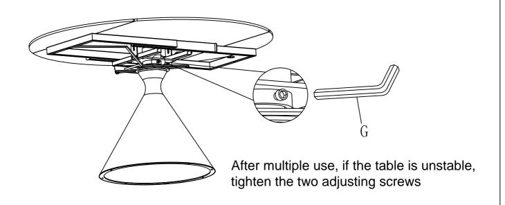
Attention! After assembled, if the top not flat, please loosen the screw and adjust the nuts till it's flat.
